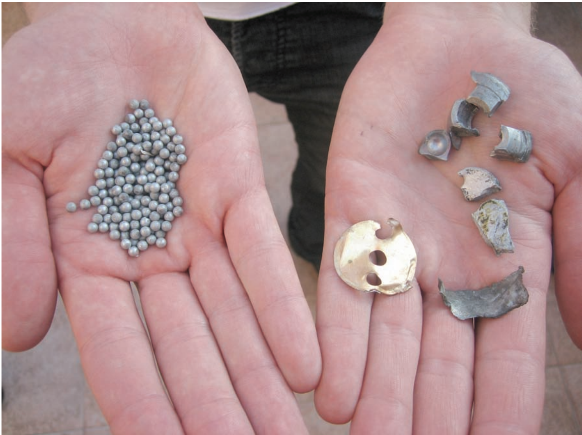
A man holds pieces of MZD-2 cluster submunitions that he said landed in his courtyard in Mghar, on July 25, 2006. On the left are the 3mm steel spheres of the type that injured three members of his family. On the right are pieces of the top of such a submunition. © 2006 Bonnie Docherty/Human Rights Watch
